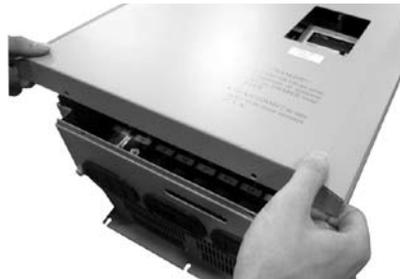
Step 2 : Carefully remove the panel
