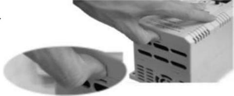
Step 2: Push to lift the lid and remove the terminal lid
