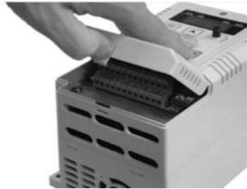
Step 3: To remove the lid for service, have both thumbs press LH & RH locking buckles to unbuckle the lid.
