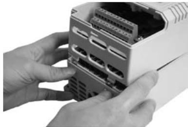
step 4: Hold and pull upward to remove the entire lid
