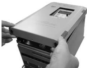
Step 1: Take and hold the PULL UP and push the panel up.
