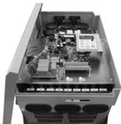
Step 1: Unscrew to remove four screws first.
