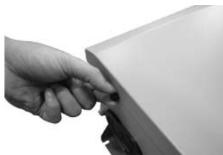
Step 1: Unscrew to remove four screws first.
